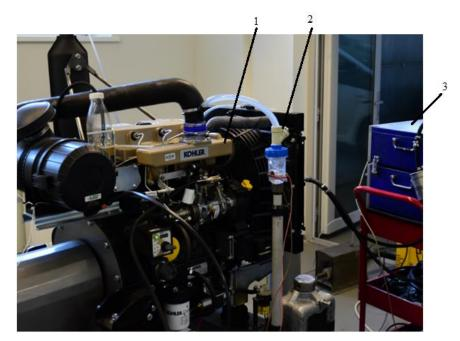
Fig. 1. **Test engine:** 1 – engine; 2 – steam generator; 3 – fuel consumption measuring equipment
