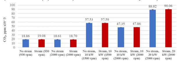
Fig. 3. CO<sub>2</sub> at different testing conditions with and without steam addition
