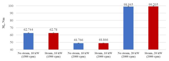
Fig. 6. Torque at different testing conditions with and without steam addition
