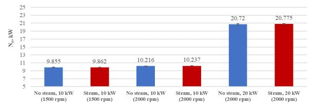
Fig. 5. Power at different testing conditions with and without steam addition
